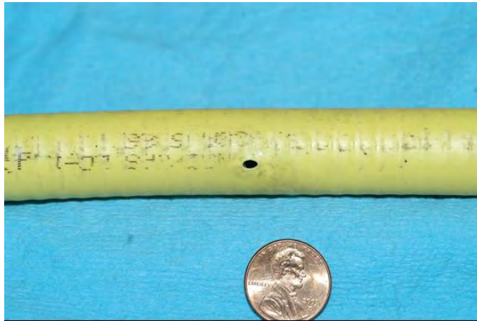
Figure 7: Photo of perforated CSST without pyrolysis
